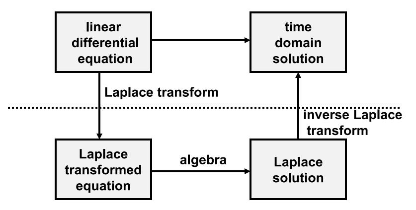
Laplace domain or complex frequency domain Basic Tool For Continuous Time: Laplace Transform
